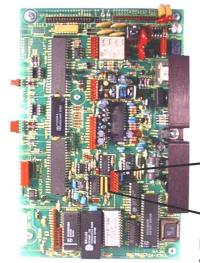
SERIAL PORT ADAPTER For communications that must occur a longer distance than 100 feet, (but less than 1000 feet) the current loop may be used instead of the RS 232 signals. The three loops supported are the busy loop, the receive loop and the transmit loop.
