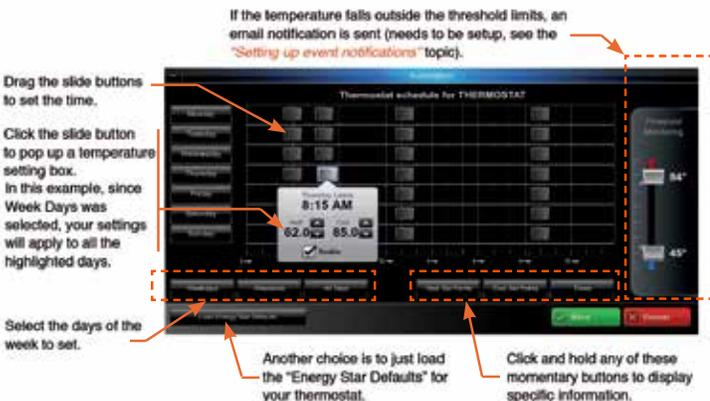
With the momentary “Heat Set Points” button depressed, the temperatures are displayed.
