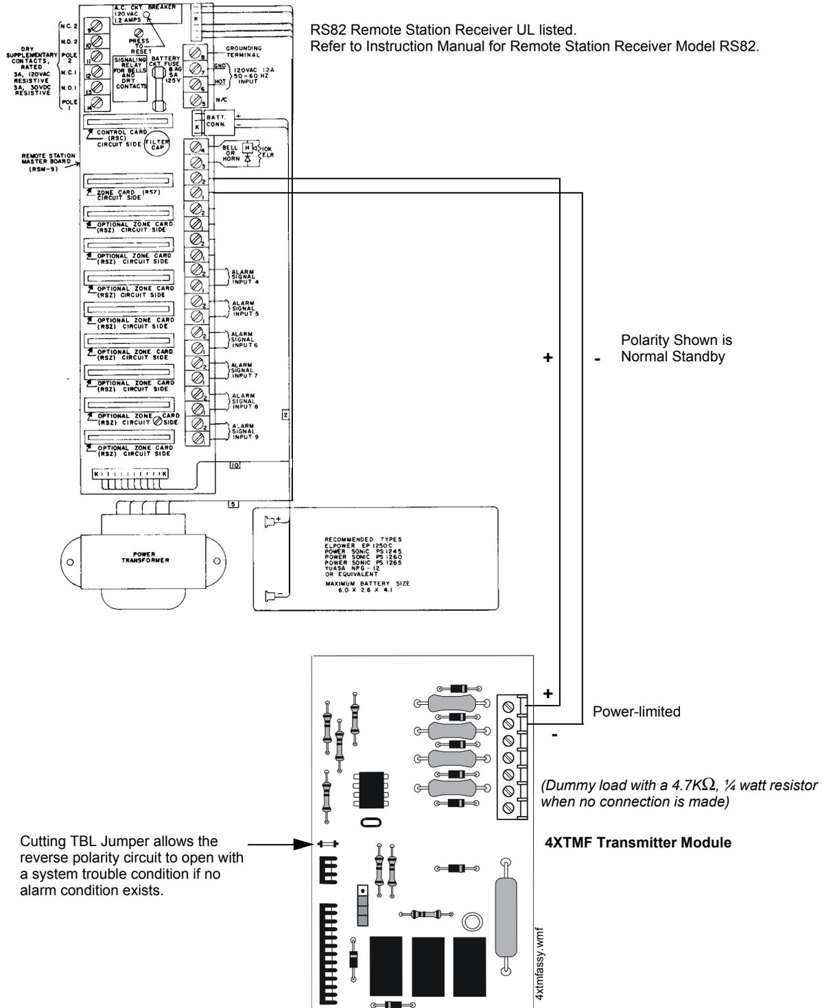
Figure C.2 Remote Station Connection Using 4XTMF Module
