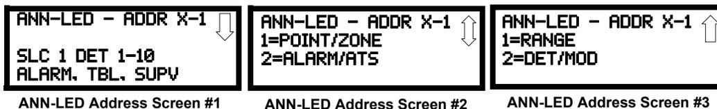
The first screen indicates that the ANN-LED at the selected ANN-BUS address is programmed to annunciate Alarms, Supervisories, and Troubles for SLC Loop #1 addressable Detectors with addresses 1 through 10. The programming can be changed using ANN-LED Address Screens 2 and 3.
