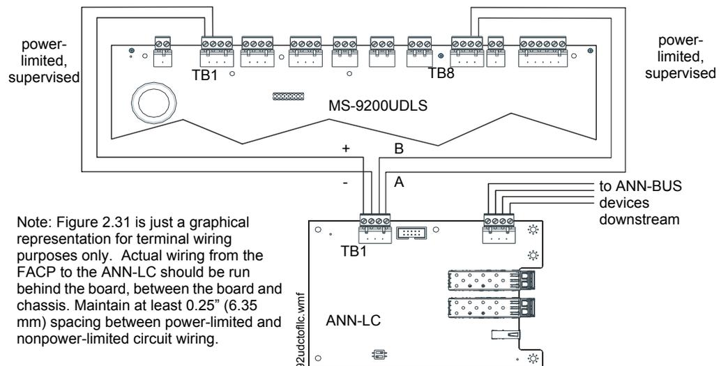
**Figure 2.31 Wiring the ANN-LC to the MS-9200UDLS**
