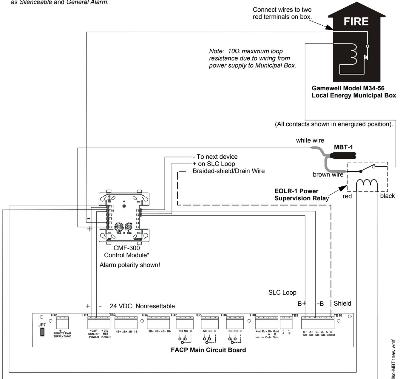
\*If the SLC device does not match the one in this figure, refer to the SLC manual wiring conversion charts for legacy and newer versions of the modules.
