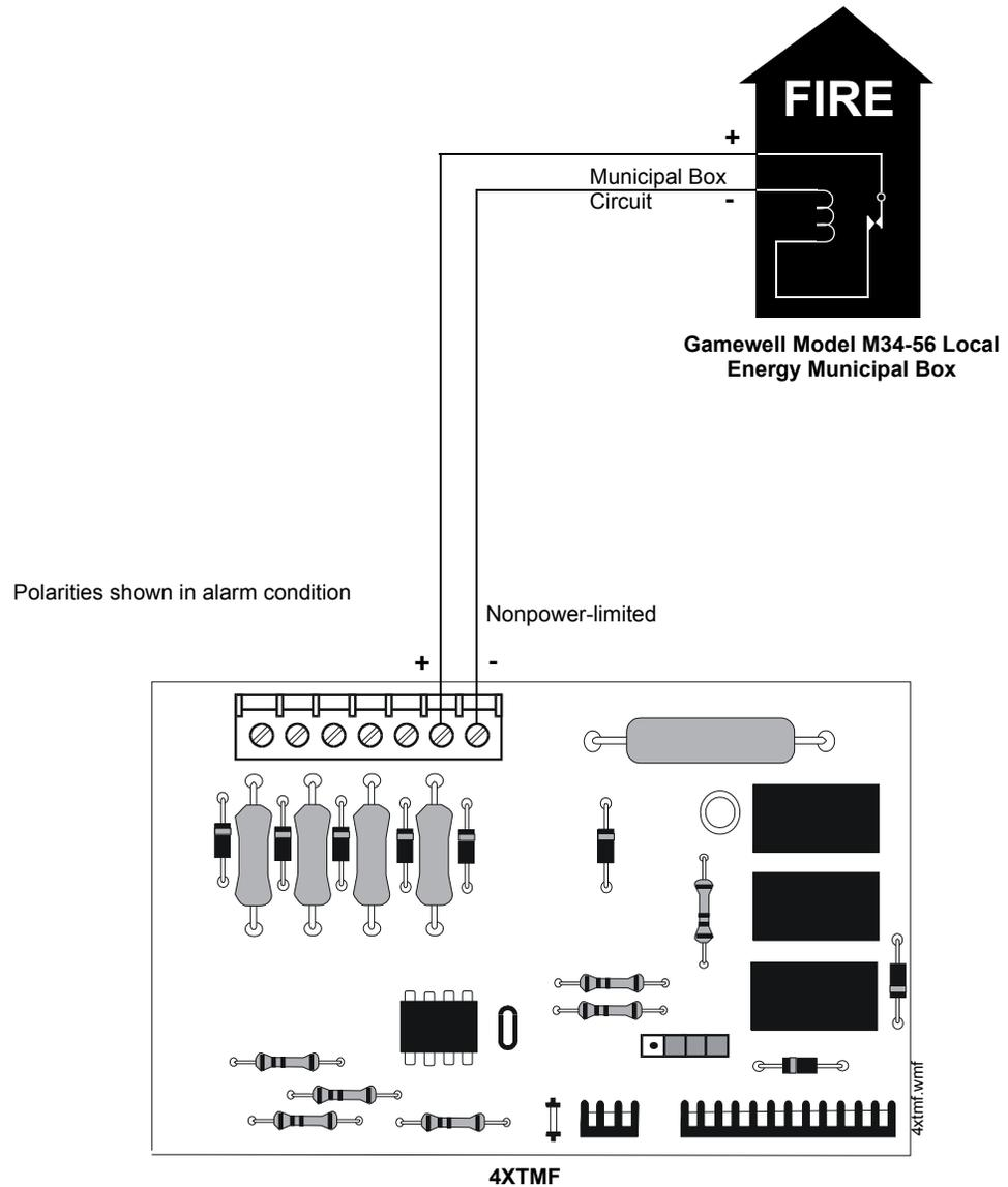
**Figure C.1 Municipal Box Connected to 4XTMF Transmitter Module**
