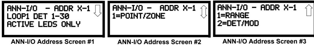
The first screen indicates that the ANN-I/O at ANN-BUS address 1 is programmed to annunciate SLC Loop #1 addressable Detectors with addresses 1 through 30. The programming can be changed using ANN-I/O Address Screens 2 and 3.
