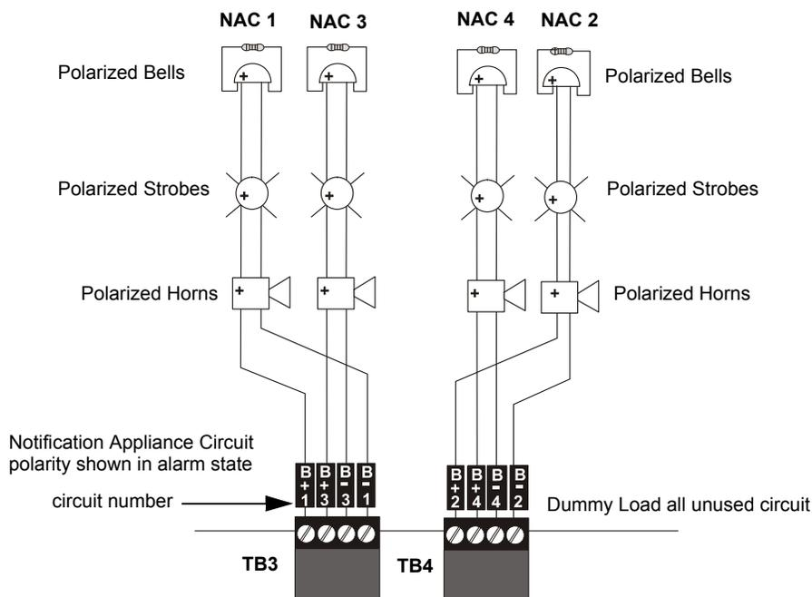
Figure 2.8 NAC Style Y (Class B) Wiring
