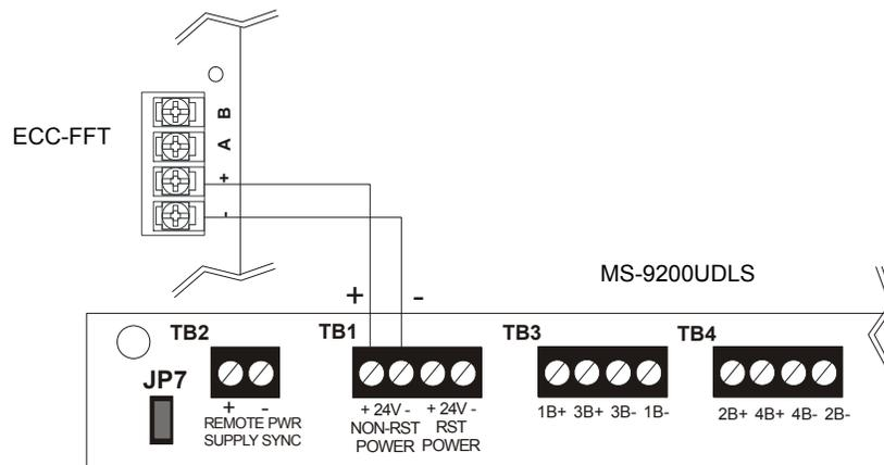
Figure 2.33 ECC-FFT Connections
