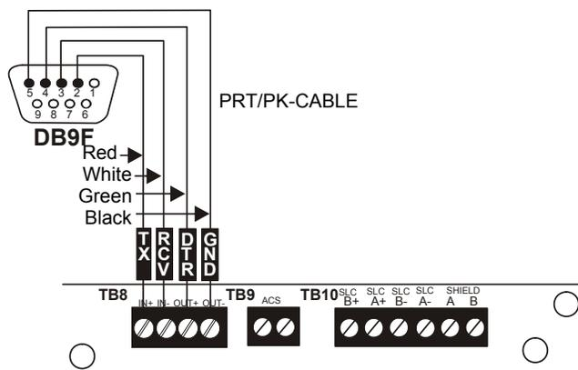
**Figure 2.32 Serial Printer and Computer Connections**
