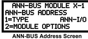
Since the options for each of these module types can be individually set, pressing 2 for *Module Options*, while viewing the ANN-BUS Address Screen will display the available options as described below.
