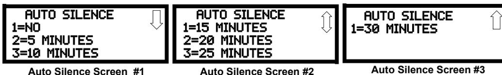
To disable the Auto Silence feature, press 1 for *No* while viewing Auto Silence Screen #1. To enable the Auto Silence feature, press the number corresponding to the time delay which will elapse before Auto Silence activates. This information will be stored in memory and the display will return to NAC Screen #2.
