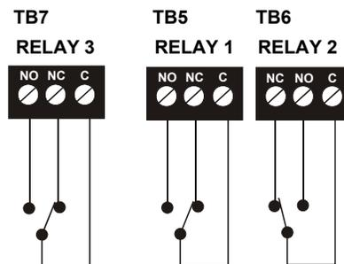
Relay contacts shown with power applied to panel and no active troubles, alarms or supervisories
