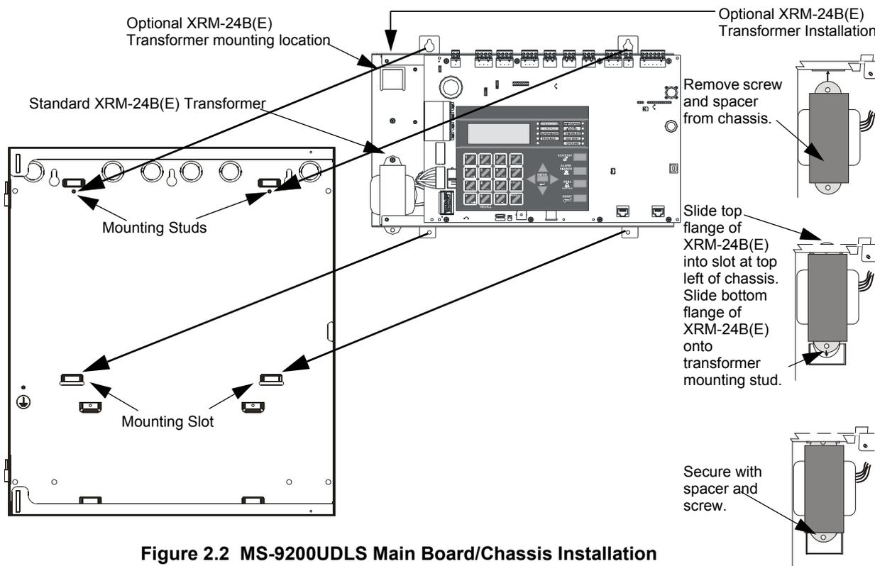
Figure 2.2 MS-9200UDLS Main Board/Chassis Installation
