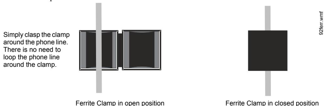
Figure 2.14 Ferrite Clamp Installation
