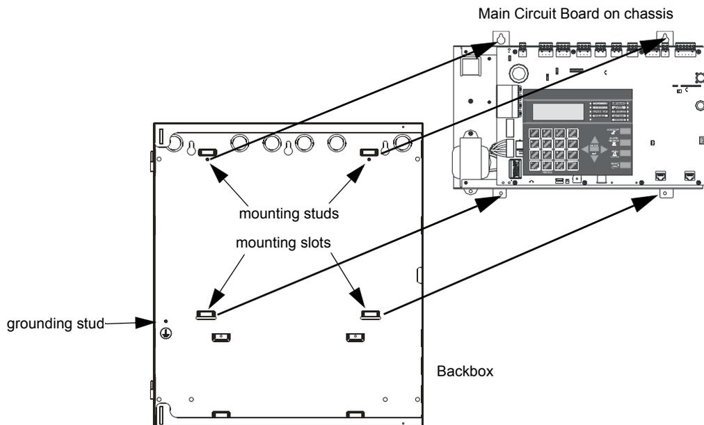
Figure 2.1 MS-920UDLS Chassis Removal
