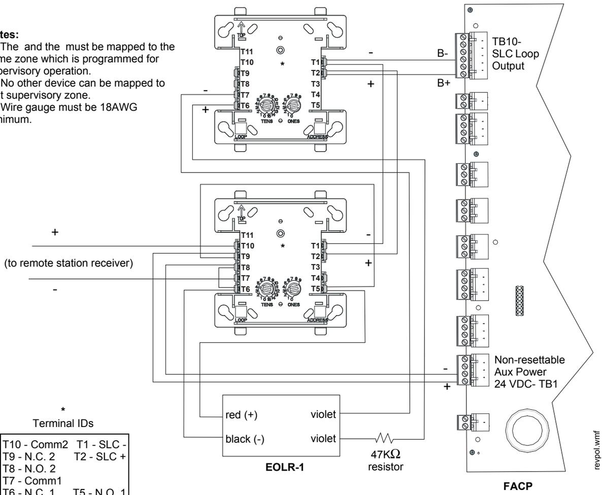
\*If the SLC device does not match the one in this figure, refer to the SLC manual appendix, which contains wiring conversion charts for type V and type H modules.
