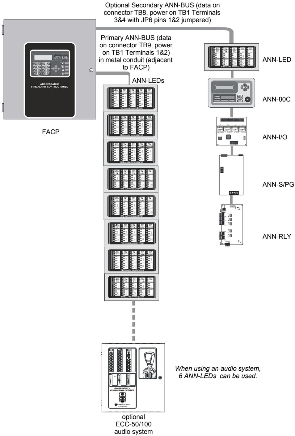
Figure I.2 FACP Maximum Configuration - Eight ANN-LEDs
