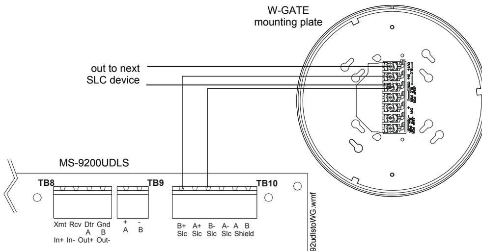
Figure 2.34 W-GATE SLC Connection
