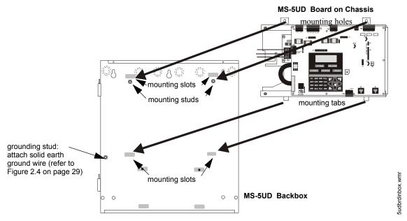
Figure 2.1 Chassis Mounting in Backbox
