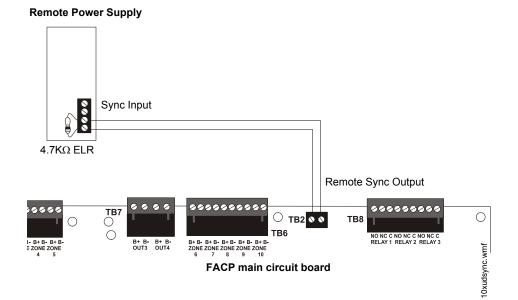
Figure 2.10 Remote Sync Output
