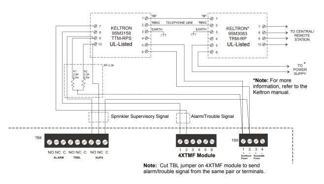
Fire Alarm Control Panel (terminal blocks are not shown in their actual positions in order to clarify wiring connections)
