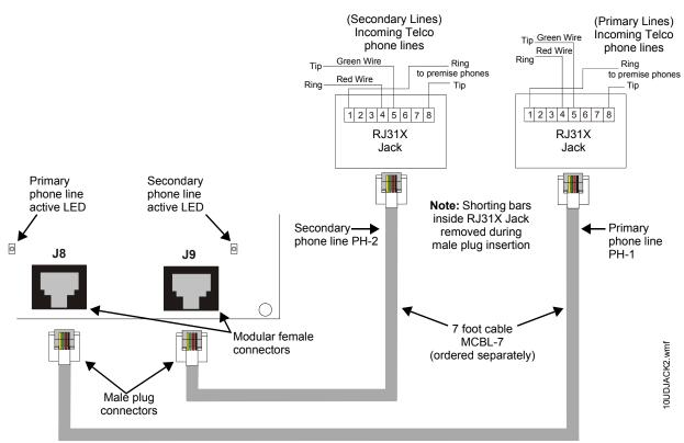
Figure 2.13 Wiring Phone Jacks
