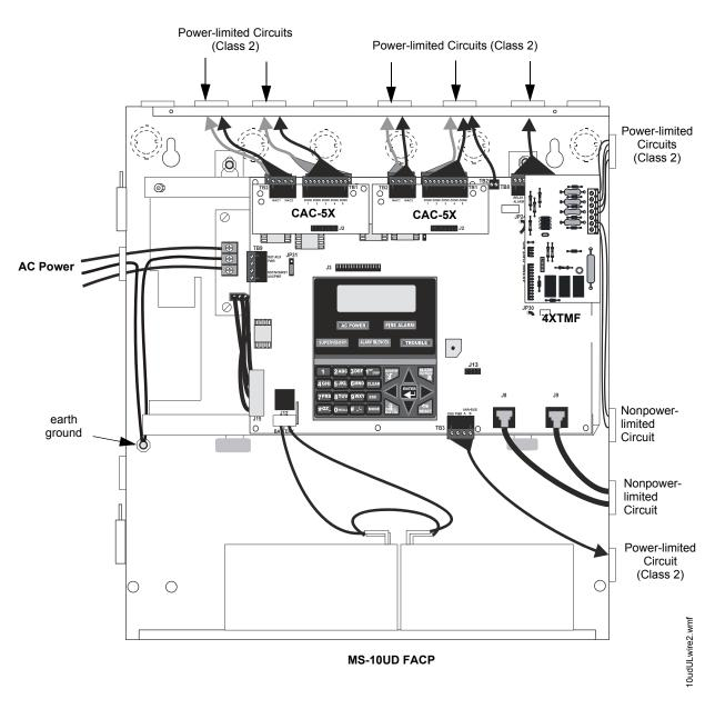
Figure 2.11 Typical UL Power-limited Wiring Requirements
