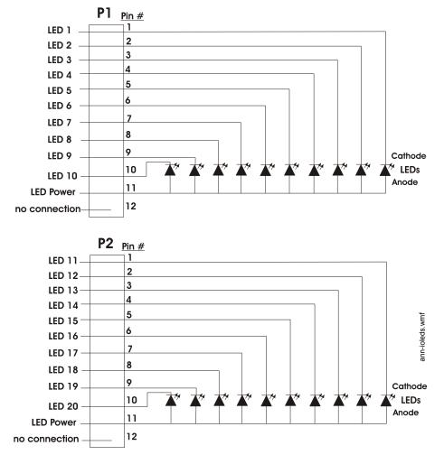
The LEDs are wired as illustrated in Figure 2.26. Note that the illustration depicts only connectors P1 and P2. Wiring is identical for P3 (LEDs 21-30) and P4 (LEDs 31-40).
