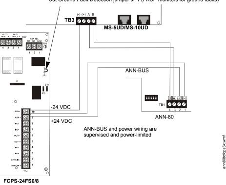
Cut Ground Fault Detection jumper JP1 (FACP monitors for ground faults)
