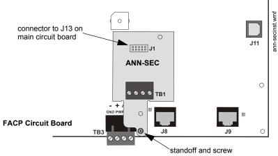
Figure 2.18 Installing the ANN-SEC Option Card
