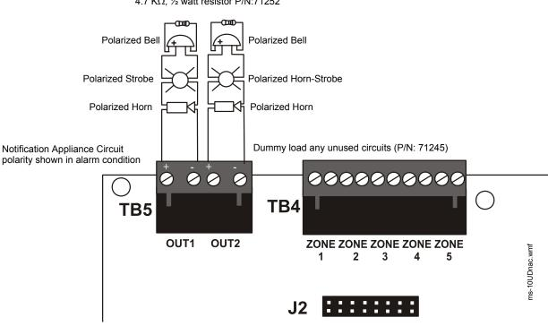
Class B Notification Appliance Circuits (supervised and power-limited) 4.7 K $\Omega$ , ½ watt resistor P/N:71252
