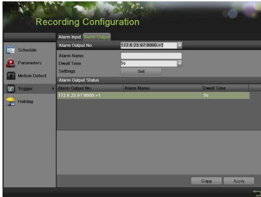
Figure 76 Alarm Output Settings Menu
