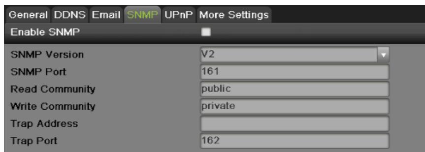
The screenshot shows the SNMP settings interface. At the top, there are tabs for General, DDNS, Email, SNMP (selected), UPnP, and More Settings. Below the tabs, there is a checkbox for 'Enable SNMP' which is currently unchecked. The settings are as follows:
