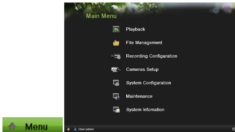
**Menu:** Click to go to NVR Main Menu. If the system is locked, you must enter the current Admin password to exit out of the Live Feed.
