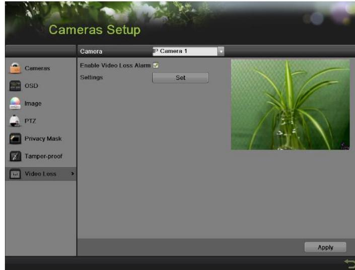
Figure 86 Video Loss Detection Menu
