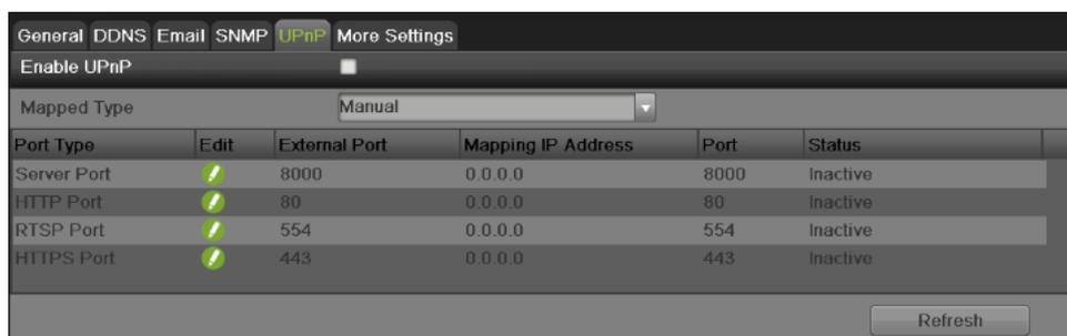
The screenshot shows the UPnP settings interface. At the top, there are tabs for General, DDNS, Email, SNMP, UPnP (selected), and More Settings. Below the tabs, there is a checkbox for 'Enable UPnP' which is currently unchecked. The 'Mapped Type' is set to 'Manual'. Below this is a table of port mappings:
