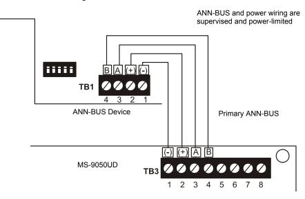
Figure 2.13 FACP wiring to ANN-BUS Device
