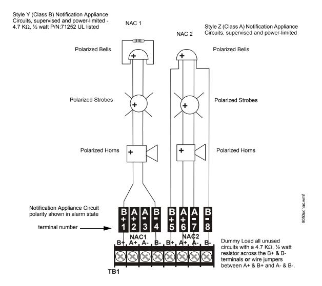
Figure 2.6 NAC Wiring
