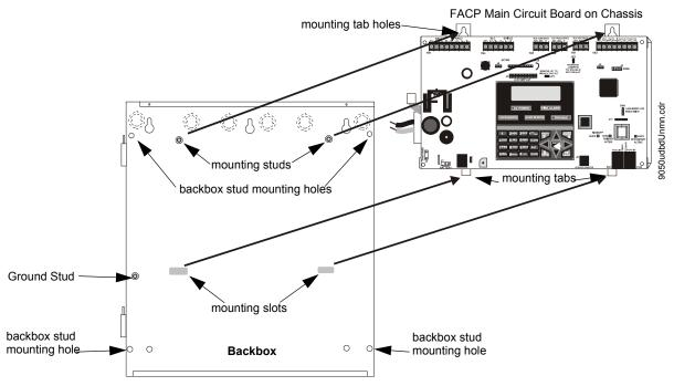
Figure 2.1 Chassis Removal
