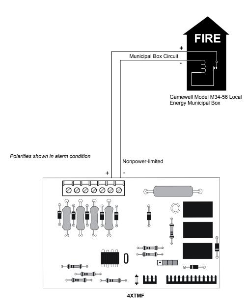
Figure C.1 Municipal Box Connected to 4XTMF Transmitter Module NFPA 72 Remote Station Protective Signaling System Notes:
