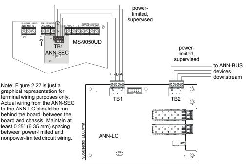
Figure 2.27 Wiring the ANN-LC to the MS-9050UD Via the ANN-SEC Card
