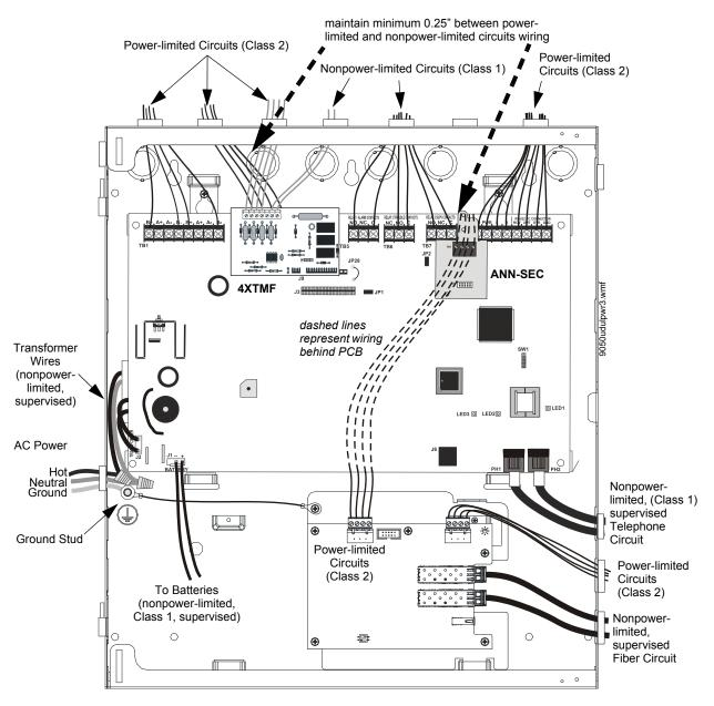
Figure 2.7 Typical UL Power-limited Wiring Requirements
