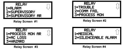
While viewing the selected screen, press the number corresponding to the desired relay type to program the main circuit board relay. The choice will be stored in memory and the display will return to the Relay Type Screen which will show the programmed type choice. Press the Escape key to return to the Relays Selection Screen and repeat the preceding procedure for the remaining relays.
