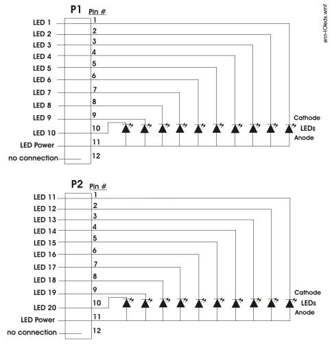
The LEDs are wired as illustrated in Figure 2.19. Note that the illustration depicts only connectors P1 and P2. Wiring is identical for P3 (LEDs 21-30) and P4 (LEDs 31-40).
