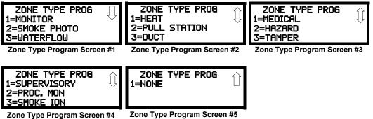
To change the zone type for Z02 to Pull Station, scroll the display until Zone Type Program Screen #2 is displayed. Press 2 to program zone Z02 as a Pull Station zone. The display will return to the Zones Installed Screen showing zone Z02 and the Pull Station program type. Repeat the procedure for each zone to be changed.
