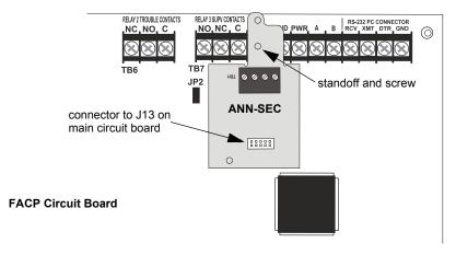
Figure 2.12 Installing the ANN-SEC Option Card
