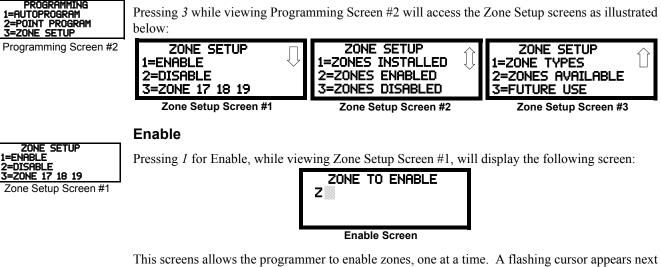
This screens allows the programmer to enable zones, one at a time. A flashing cursor appears next to the Z, prompting the programmer to enter a two digit zone number (01 - 19). When the second digit is entered, the zone will be enabled and the cursor returns to the original position next to the Z. Another zone can then be enabled.
