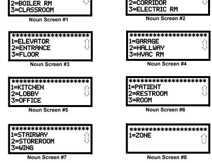
Pressing 3 or 4 while viewing the Adjective/Noun Screen will display screens similar to the previous Adjective and Noun Screens. The new screens will list Custom Adjectives and Nouns which have been programmed into the control panel using the PK-CD. These descriptors are selected as described in the previous sections.
