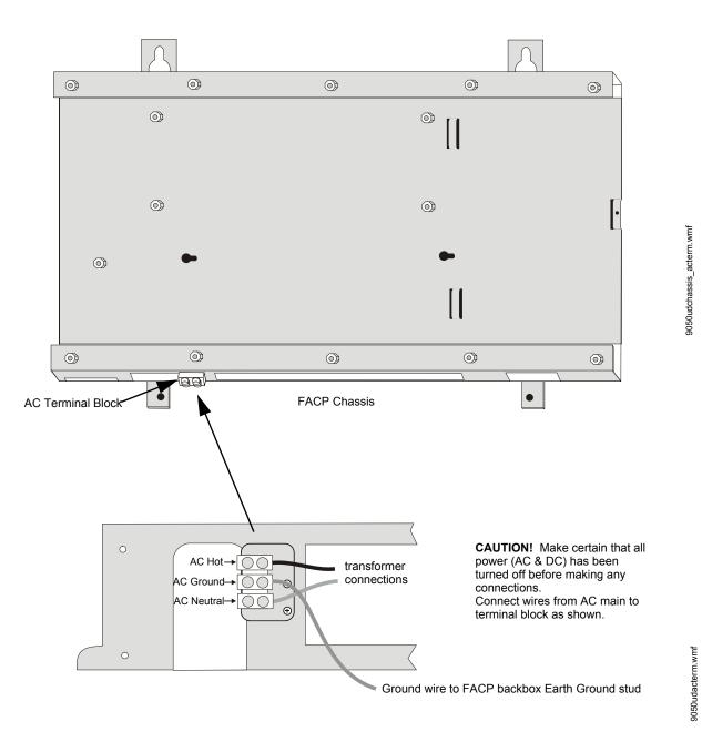
Figure H.4 AC Terminal Block Connections
