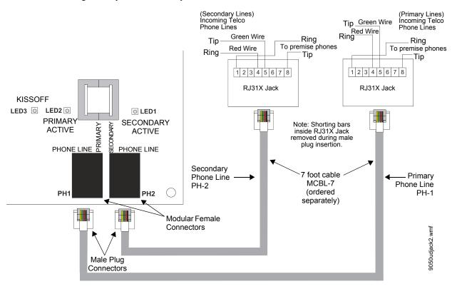
The control panel's digital communicator is built into the main circuit board. Connection and wiring of two phone lines is required as shown below.
