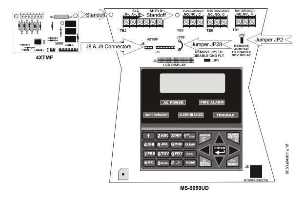
Figure 2.11 4XTMF Connectors to MS-9050UD Connectors
