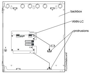
Figure 2.25 Mounting the ANN-LC into the Backbox
