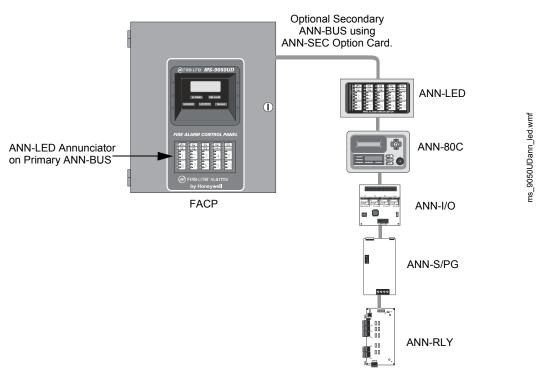
Figure H.1 FACP Minimum Configuration - Single ANN-LED Annunciator
