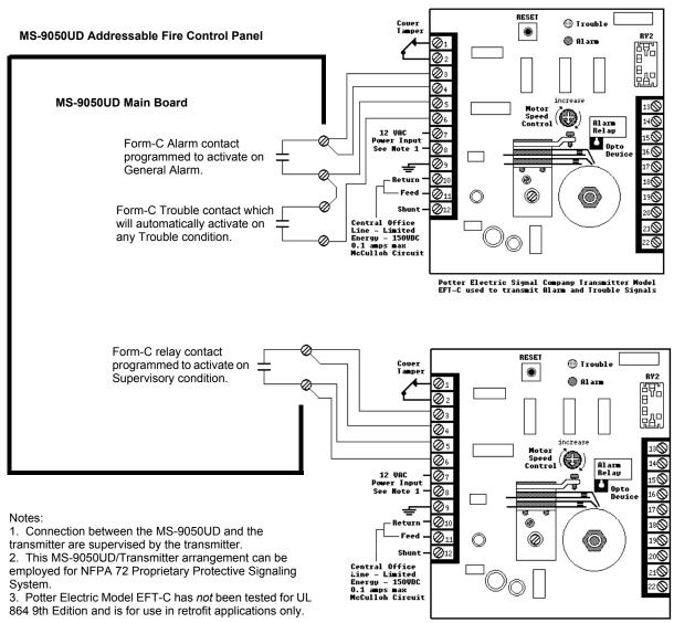
Potter Electric Signal Company Transmitter Model EFI-C used to transmit Alarm and Trouble Signals
