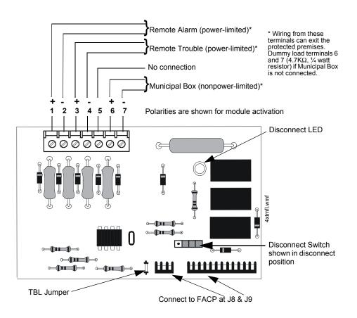
Figure 2.10 4XTMF Transmitter Module
