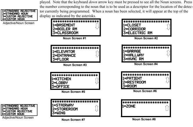
Pressing *3* or *4* while viewing the Adjective/Noun Screen will display screens similar to the previous Adjective and Noun Screens. The new screens will list custom Adjectives and Nouns which have been programmed into the control panel by the user utilizing the PK-CD programming kit. These descriptors are selected as described in the previous sections.
