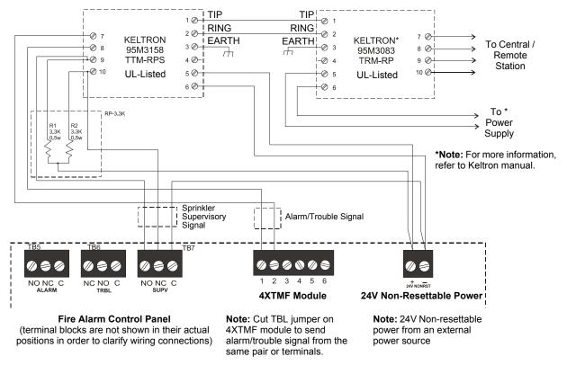
Figure D.1 FACP With Keltron Wiring
