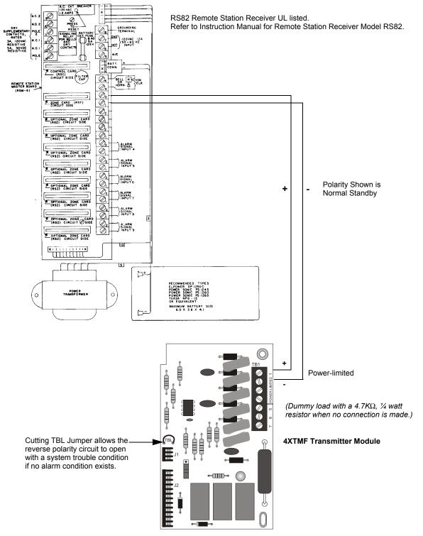
Figure C.2 Remote Station Connection Using 4XTMF Module
