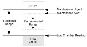
Figure 4.1 Diagram of Maintenance Levels
