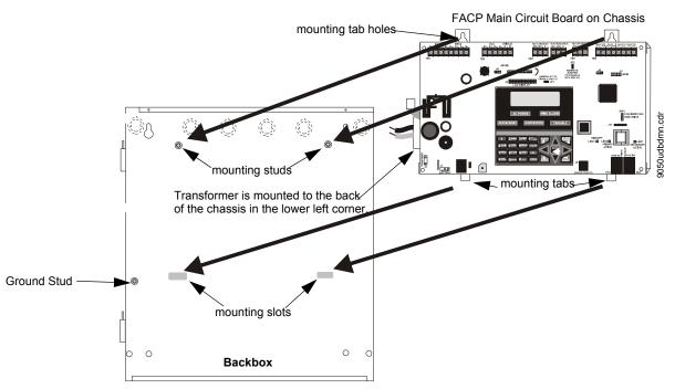
Figure 2.2 Main Circuit Board/Chassis Installation
