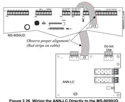
Figure 2.26 Wiring the ANN-LC Directly to the MS-9050UD
