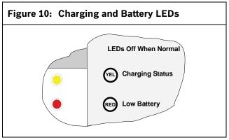
**Investigate Low Battery reports immediately:** If primary (AC) power is off and the discharge continues, the control panel becomes inoperative when the battery voltage drops below 10.2 VDC.
